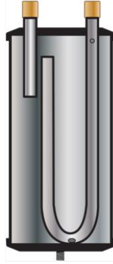
Figure: Cross section of accumulator
